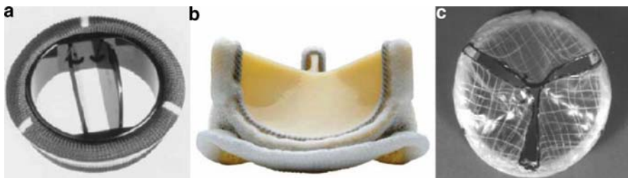
Fig. 14 Artificial heart valves: Bileaflet mechanical valve (a) [22], bovine pericardial bioprosthetic valve (b) [47], synthetic valve with sinusoidal fiber reinforcement (c) [14]
