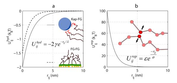
**Figure 5. The nonbonded potential energies employed in the model. a**) Hydrophobic potential energy is applied between FG-beads localized to the central channel (dashed line). The same potential, a bit stronger, is applied between kap and FG-beads (solid line). **b**) Pairwise repulsive potential. doi:10.1371/journal.pcbi.1002049.g005
